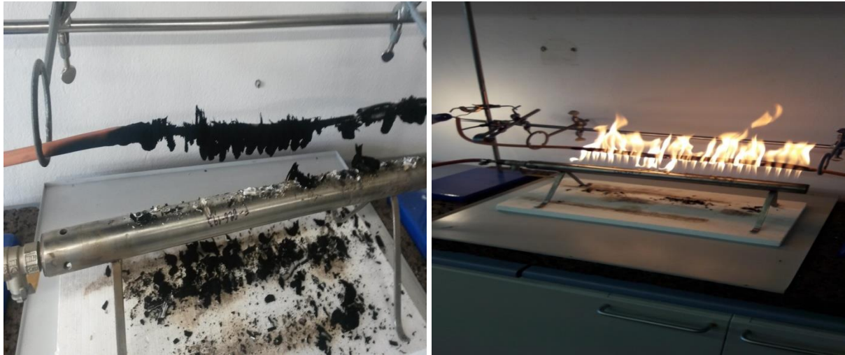
Fig. 1. Test of circuit integrity of cable according to STN IEC 60331-21 [9]
