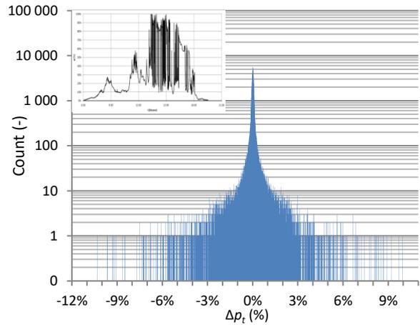
Figure 7. Statistical frequency of power changes in 1 second period—partly cloudy (PVPP no. 2)
