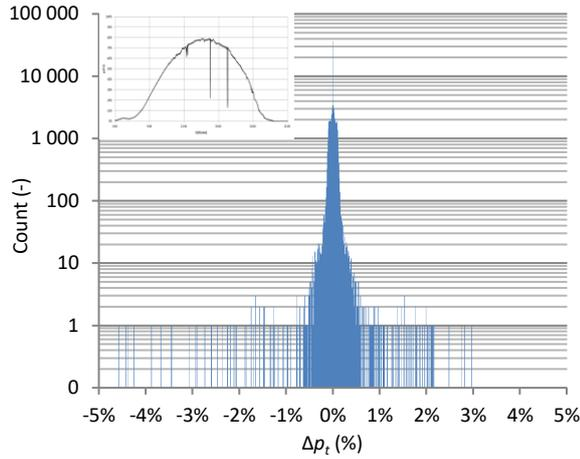
Figure 4. Statistical frequency of power changes in 1 second period—sunny day (PVPP no. 1)
