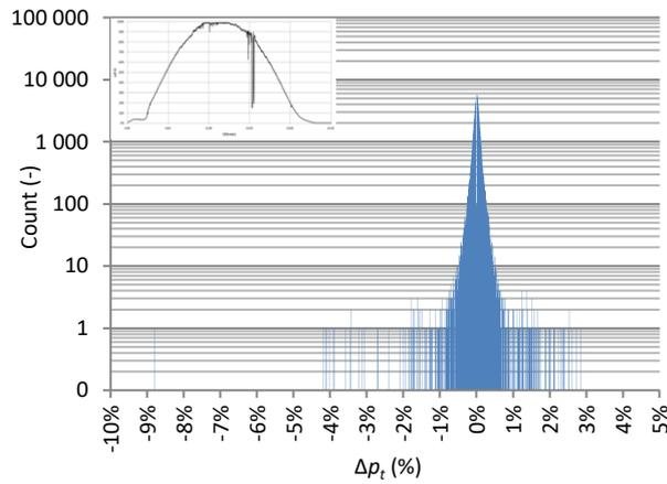
Figure 5. Statistical frequency of power changes in 1 second period—sunny day (PVPP no. 2)
