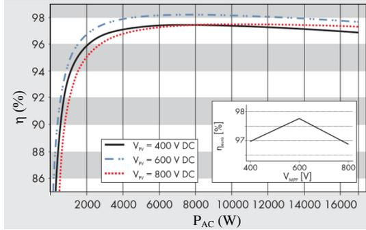
Figure 3. Efficiency dependence on produced power of inverters used for PVPP no. 2
