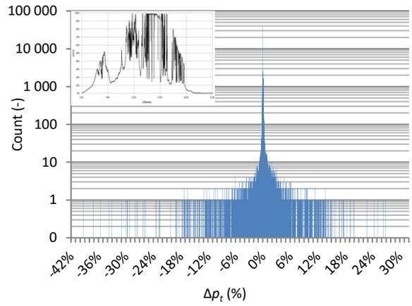
Figure 6. Statistical frequency of power changes in 1 second period—partly cloudy (PVPP no. 1)
