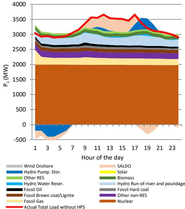
Figure 1. Daily diagram of system load at day with minimal production of PVPP (24.12.2021)[8]
