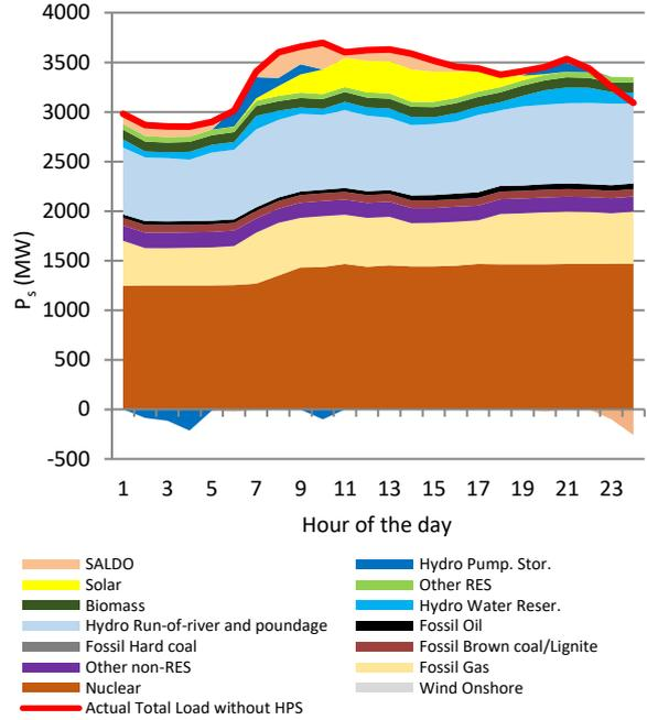
Figure 2. Daily diagram of system load at day with minimal production of PVPP (26.05.2021)[8]
