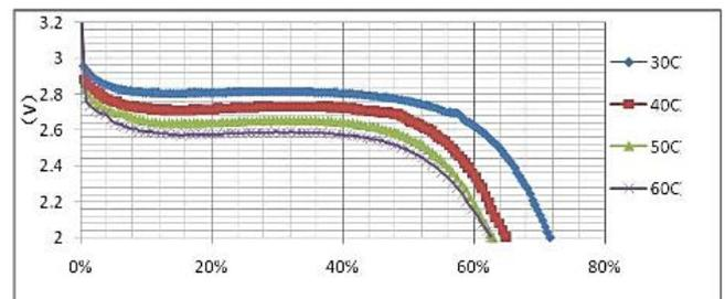
Fig. 1. The discharging chart of LiFePO<sub>4</sub> battery cell [3]
