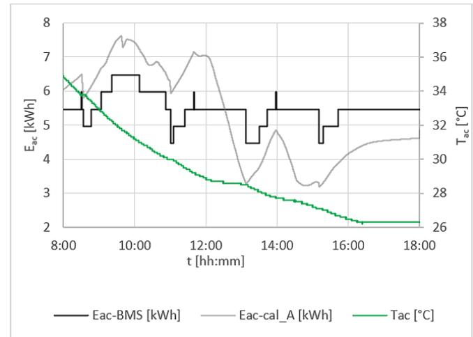
Fig. 10. The curve of stored energy on workday - consumption balancing.
