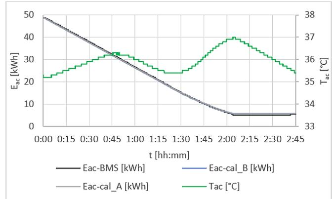
Fig. 9. The curve of stored energy at -20,2 kW discharging power ( $P_{ac} = -22,6$  kW)
