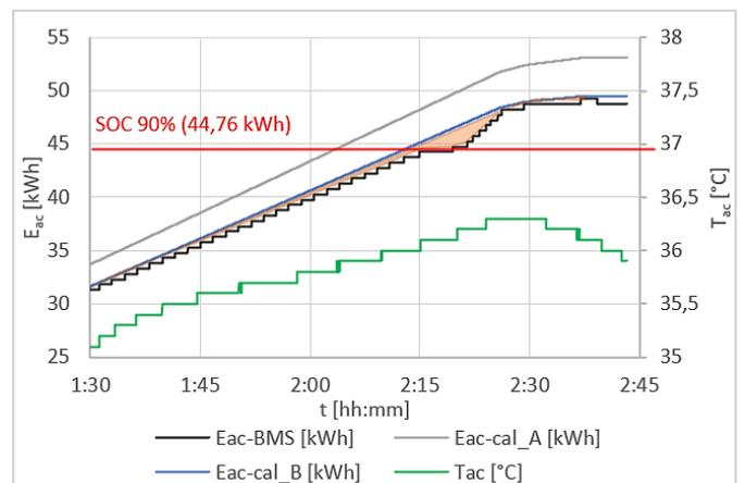
Fig. 7. The curve of stored energy at 21,1 kW charging power ( $P_{ac} = 17,9$  kW,  $P_{cor} = 1,4$  kW)
