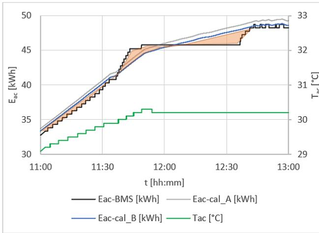
Fig. 10. Fig. 11. The curve of stored energy on weekday - consumption balancing.
