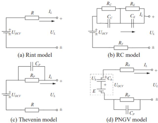
Fig. 2. The most simple equivalent batteries circuit schemes [4]
