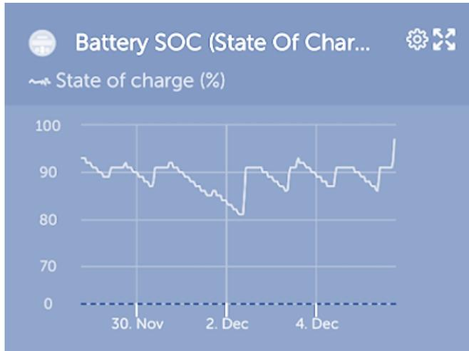
Fig. 4. SOC curve of BESS in users application [7]
