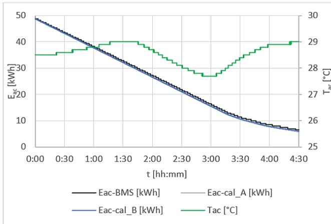
Fig. 8. The curve of stored energy at -10,3 kW discharging power ( $P_{ac} = -11,1$  kW)
