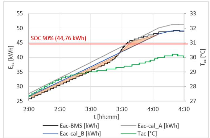
Fig. 5. The curve of stored energy at 11,2 kW charging power ( $P_{ac} = 10,2$  kW,  $P_{cor} = 1,4$  kW)
