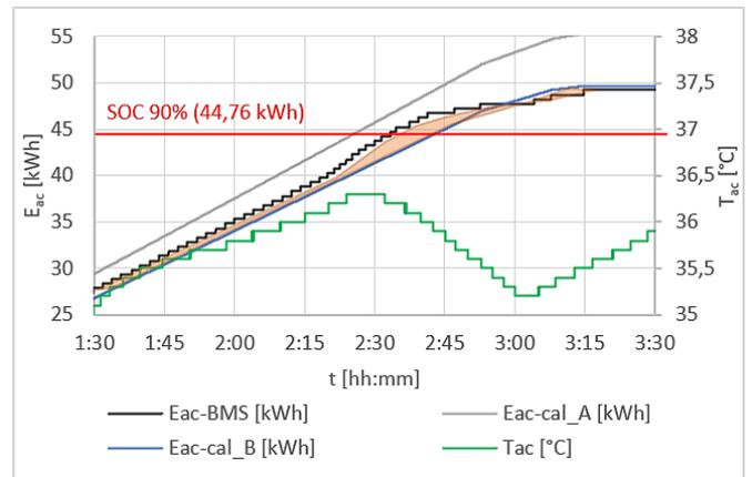
Fig. 6. The curve of stored energy at 17,4 kW charging power ( $P_{ac} = 14,4$  kW,  $P_{cor} = 1,4$  kW)
