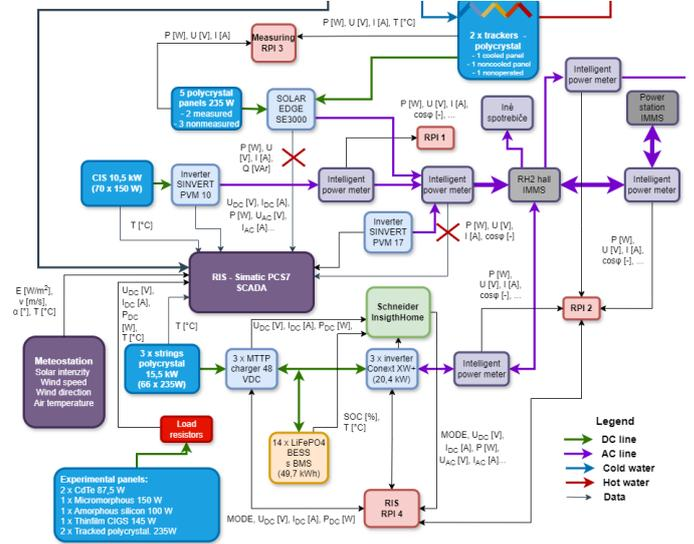
Fig. 3. Block diagram of the connection and devices IMMM SAS ENERGY HUB
